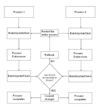
Depending on the size of the datasource for Process 2, the data rollback and process re-execution can cause a noticeable decrease in performance. To address this performance issue, consider using the BatchUpdateFinishWait function in place of BatchUpdateFinish.
